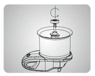
Remove the Spring from Grinder Shaft
