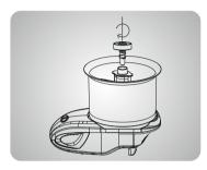
Fix the Spring and tighten (clock wise) properly
