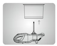
Remove the Roller from Drum Remove the Drum from Grinder
